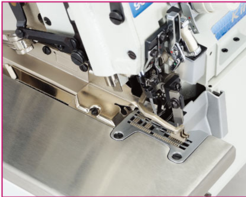
US040:側吸風式自動切線刀(水平吸風式) Side suction type thread trimmer (horizontal type).
